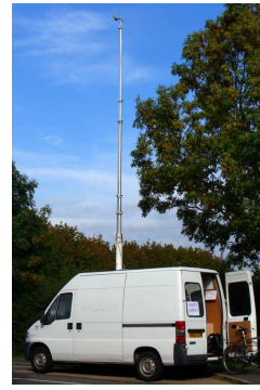
Fig. 2. The IRISYS infrared sensor being used to count cars in Cambridge, October 2006. The sensor is the small box at the top of the van's erectable mast.
