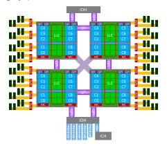
Figure : Intel Xeon Westmere E74 4 node, 10 core system
