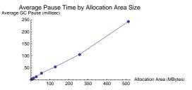
Figure : Average GC pause time for different allocation areas (generation 0) when running the local learning controller with 40 cores and 500 switches.
