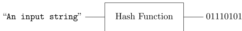
Figure 3.9: The hash function assigns a pseudo-random fixed-length string of bits to an arbitrary length input text string.
