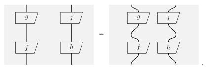
The pictorial presentation of the definition makes many of the conditions really easy to grasp. Because of the pictures, the composition of arrows is sometimes called *sequential composition* while the monoidal product is called *parallel composition*. In this thesis, as we are dealing with mostly diagrams, we will use the word 'plugging' for the sequential composition, and the word 'juxtaposition' for parallel composition.
