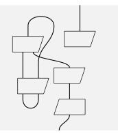
The punchline of a string diagram is that we are allowed to deform the wires, rotate the boxes, move them freely on the surface of a plane, as long as the input and output wires are in the proper order. This is the background of all the diagrams in the subsequent parts of the thesis.
