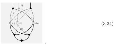
where, for i = 1, ..., m and j = 1, ..., n, the dotted wire connecting the *i*-th white vertex to the *j*-th output is present if and only if  $b_{ij} = 1$ .
