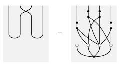
Just some remarks of the proof. We relied heavily on the bialgebra equations 2(h), 3(d) which allows us to move the monoid and comonoid pass each other. For this reason, it is believed that the Hopf algebra structure of the black vertices is a more crucial defining feature of the pure fragment of the ZW calculus than the anti-special commutative Frobenius algebra.
