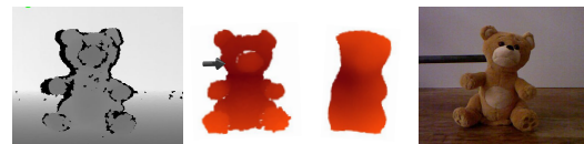
Figure 9: Cross-category prediction on a real object. Left: depth input image; middle: input voxel and predicted deformation; right: actual deformation.
