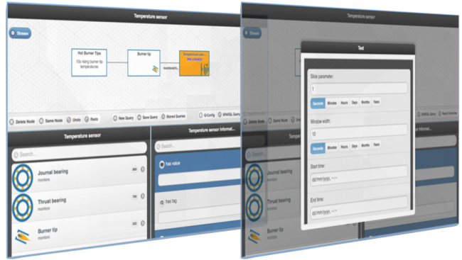
Figure 2: Example monitoring task in STARQL (on the left) and STREAMVQS (on the right)
