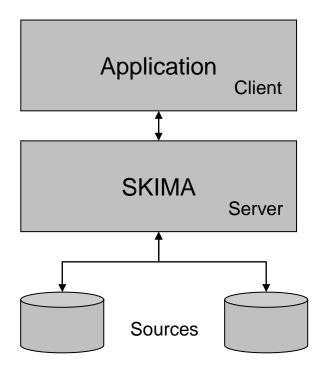
Figure 3.17 An application using SKIMA based on a client/server architecture.
